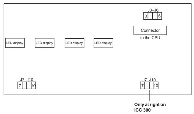
Two blocks are available to receive jumpers: At the top right is a block with the slots J3–J6, at the bottom left (ICC 300: bottom right) is the block with the slots J7–J10.
