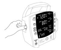
3.Place the roll of paper into the compartment so that the end of the paper comes off the right-side of the roll (paper is wound around the roll clockwise). Push the roll all the way to the back of the printer cavity, making sure the paper extends out of the printer cavity at least two inches.
