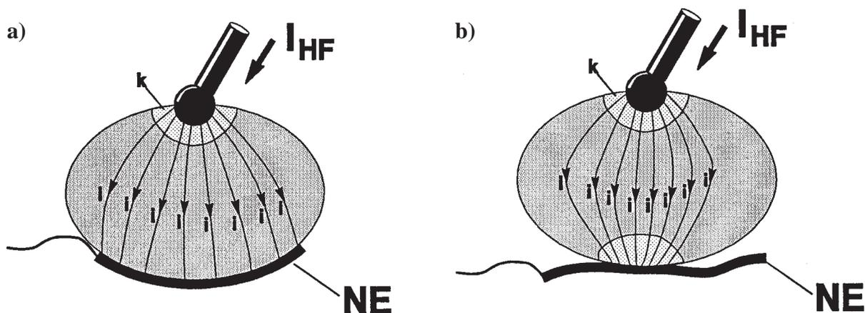
**Fig.:** The neutral electrode must be applied at an appropriate location on the patient's skin using the entire contact surface available (a). If the neutral electrode has only partial contact to the patient's skin (b), there is a risk that burning will occur at this location
