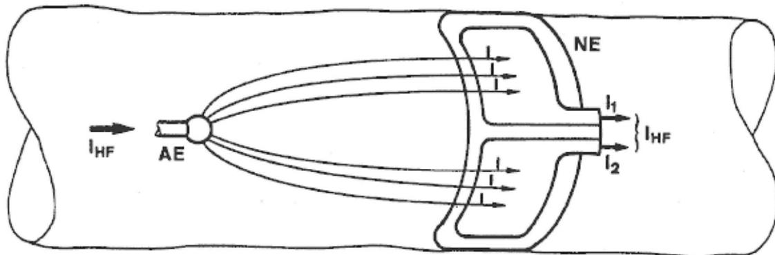
Neutral electrode suitable for NESSY - applied correctly
