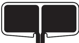
When using neutral electrodes with two contact surfaces, not only the electric connection between the unit and neutral electrode is automatically monitored, but also the application of the neutral electrode on the patient. Here the electric conductance between the two contact surfaces on the neutral electrode and the skin of the patient is constantly measured automatically and compared with the intensity of the high-frequency current that flows through the neutral electrode.
