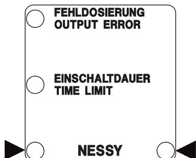
The units in the ERBOTOM ICC model series are equipped with a Neutral Electrode Safety System (NESSY), which monitors both the electric connection between the unit and neutral electrode as well as the correct application of the neutral electrode on the patient.
