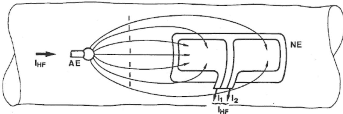
Neutral electrode suitable for NESSY - applied incorrectly
