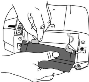
6. Then replace the cover, help card tray, and screws. Insert the external DC power converter plug into the external DC power socket and plug into an AC outlet.
