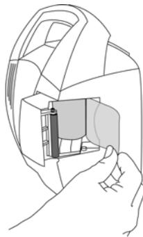
3. Place the roll of paper into the compartment so that the end of the paper comes off the right-side of the roll (paper is wound around the roll clockwise). Push the roll all the way to the back of the printer cavity, making sure the paper extends out of the printer cavity at least two inches.
