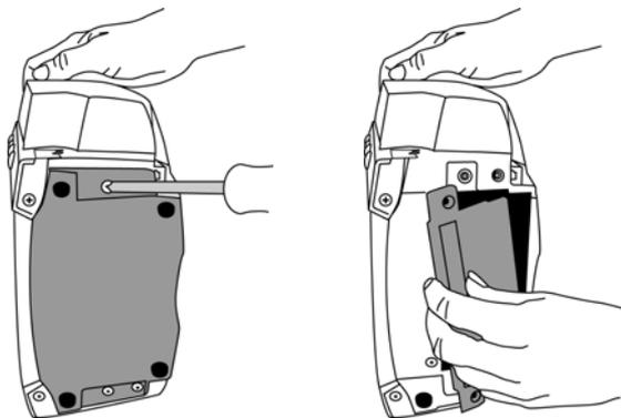
4. Remove the old battery and disconnect the wires. Attach the battery wires to the new battery, ensuring the red terminal (+) is connected to the red wire and the black terminal (-) is connected to the black wire.
